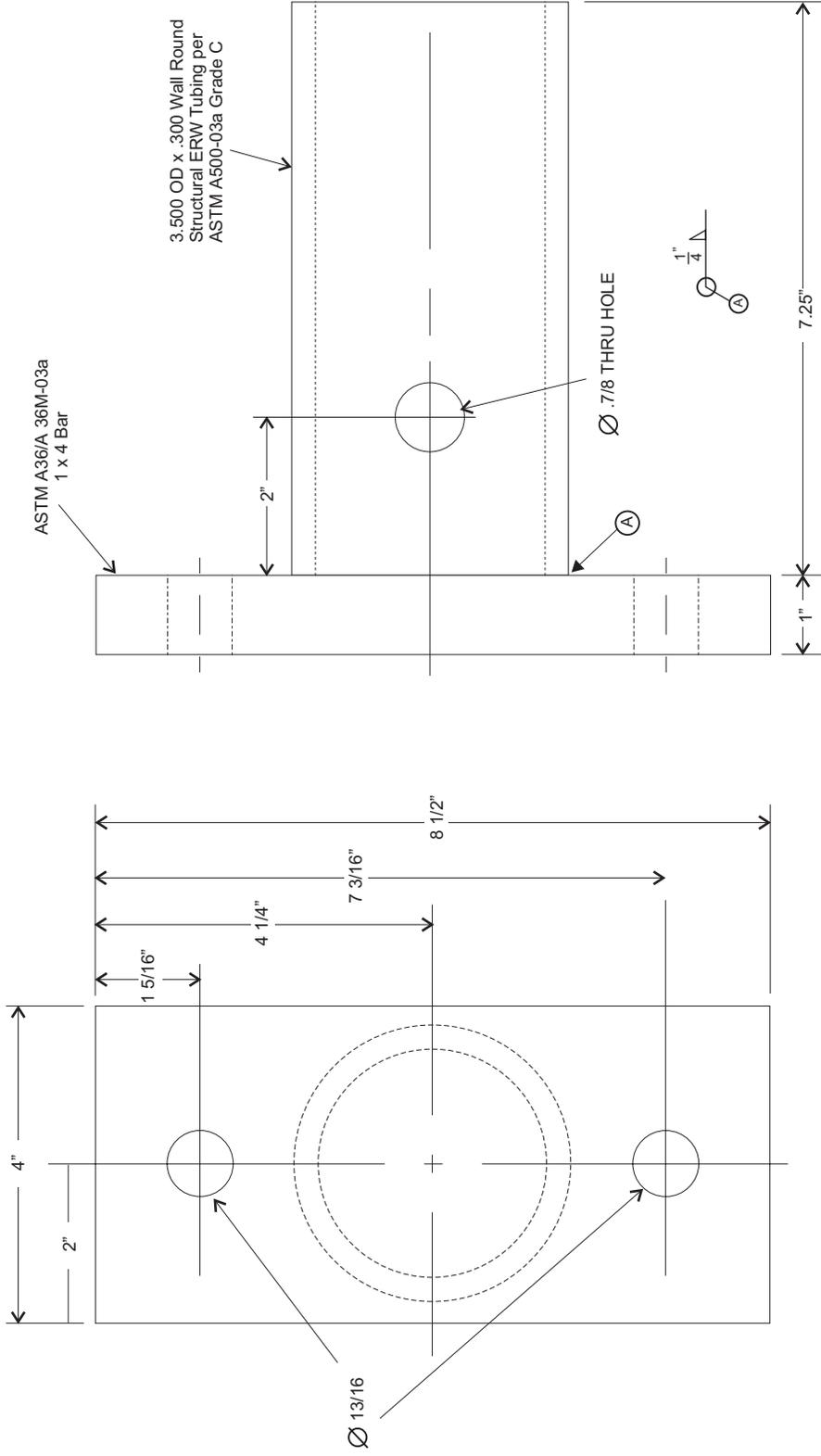
Weld: Minimum Tensile 70,000 psi
